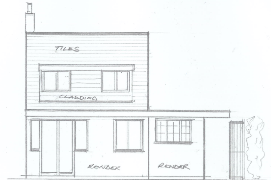
EXISTING REAR ELEVATION
